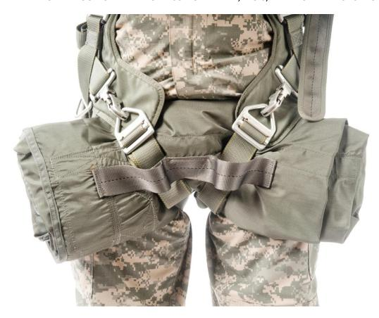
The Airborne Soldier will wear the UPKB so that the leg strap retainer is facing out and both left and right leg straps are routed from bottom to top behind the leg strap retainer. The quick fit V-ring is securely fastened to the quick ejector snaps ensuring the ejector snap activating level is secured and seated properly.
